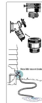
There are also devices called hose bib vacuum breakers that can be installed on your hose bib that will add protection. Hose bib vacuum breakers are fairly inexpensive, less than \$10 at the hardware store. These devices consist of a spring-loaded check valve that seals against an atmospheric outlet when the water supply is turned on.
